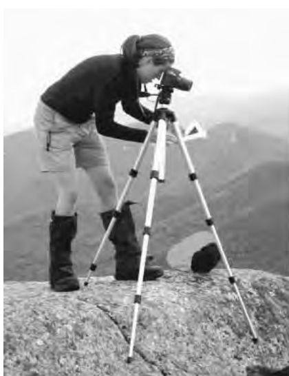
Figure 6 —Summit steward Lynn Metcalf compares the view in front of her with a print of an earlier photo point to properly line up the image. Photo courtesy of the AHPSSP.
