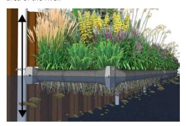
Installation took just 3 days, in collaboration with Land & Water Services and Terraqua Environmental Solutions. Sections fit together using a locking stainless steel quick connect system, which can be adjusted to match up to the curvature of the embankment.
