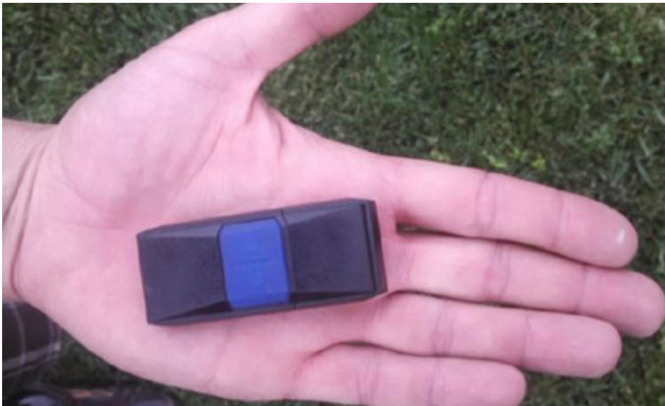
Figure 1 -The Canmore GT-740FL Sport GPS data logger with hand for scale.
