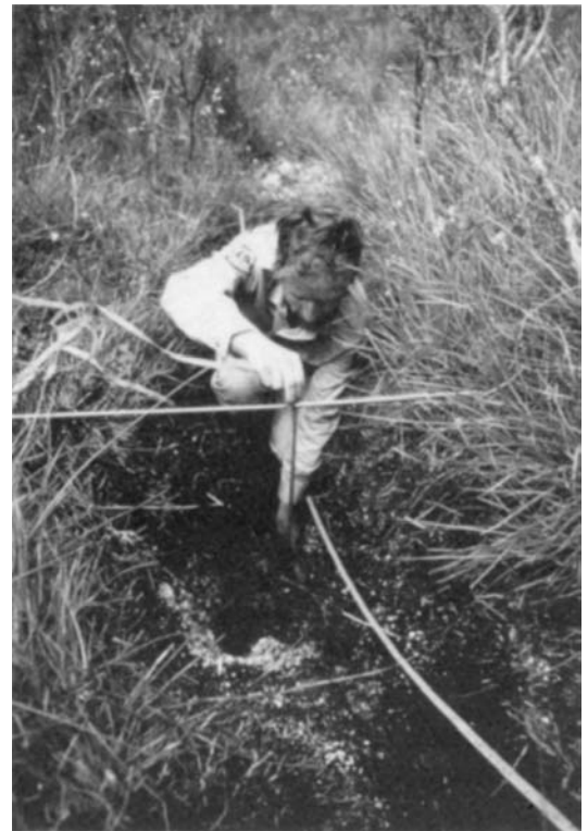
Parks and Wildlife Service officer taking measurements at one of the 400 or so monitoring sites throughout the World Heritage Area. At each site PWS officers gather information including, the depth of erosion, the loss of vegetation cover, the presence or absence of mud and the evidence of water flow. The monitoring program provides the basis for a systematic assessment of the levels, rates of change and distribution of track impacts. Photo by Tracey Diggins.
