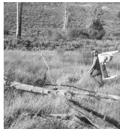
Figure 2—The Manual Wire Roller can hold 90 pounds of rolled wire equal to 1/4 mile, which is easily and efficiently rolled by the operator. Photo by John Witzel.
