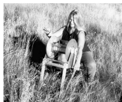
Figure 3—Here Cindy Witzel cranks in removed barbed wire onto the Steens Manual Wire Roller. Photo by John Witzel.
