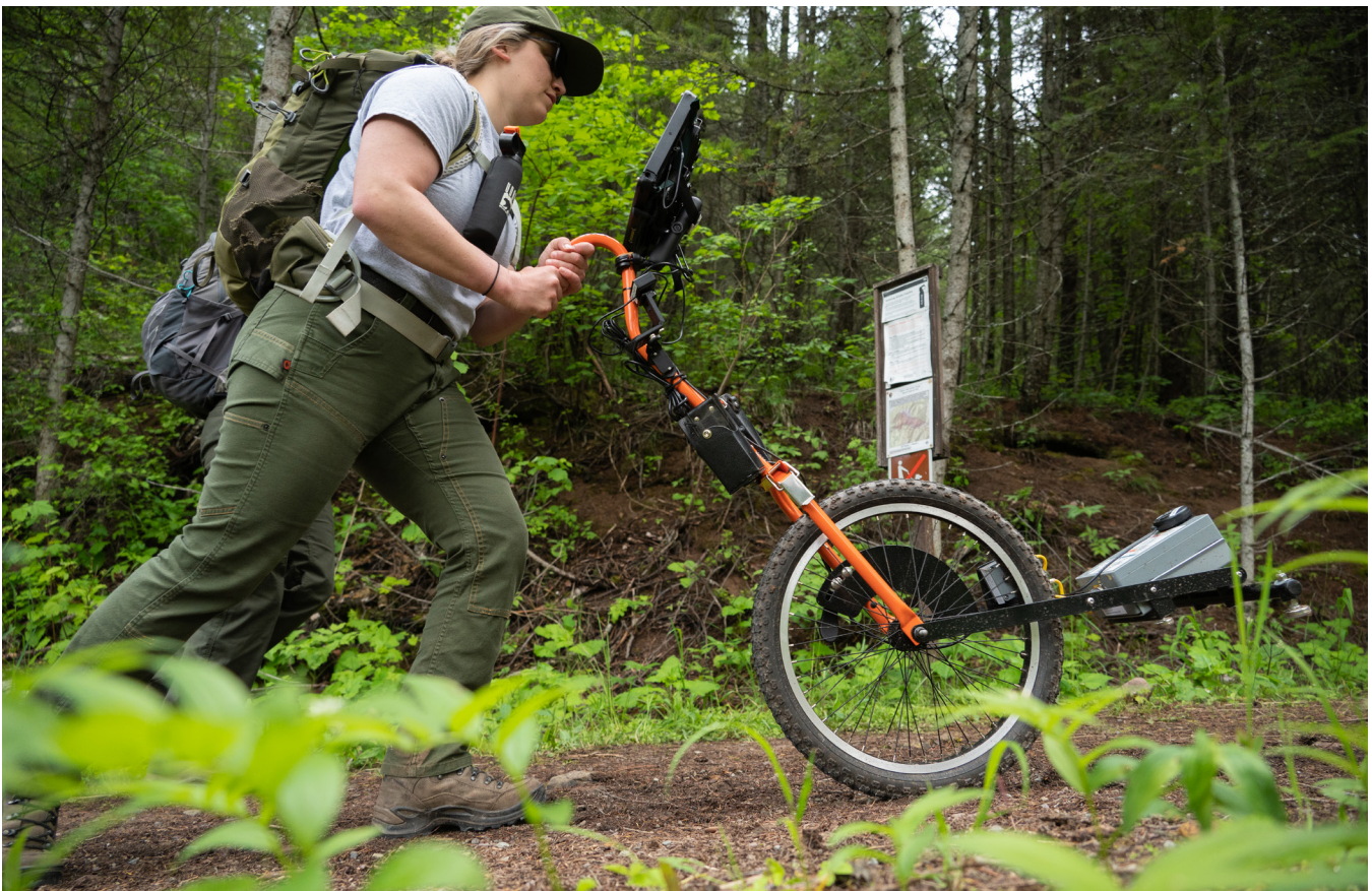
Figure 3 - The High-Efficiency Trail Assessment Process (HETAP) machine measures trail attributes that can affect a user's ability to navigate the trail. Credit: National Park Service.
